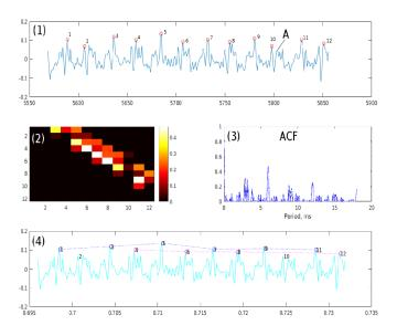
Fig. 2. Illustration of click tracking using a section of data from RATS "H" channel. (1) LPETS envelope with detections, (2) normalized ACF values for each detection pair, (3) normalized ACF, (4) LPETS envelope with associated detection groups.
